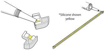
5. Carefully add the siliconed strip into position, as shown. Make sure the end caps touch up to the inline panel and the the fixed panel.
