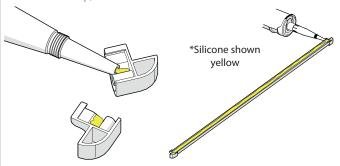
5. Carefully add the siliconed strip into position, as shown. Make sure the end caps touch up to the inline panel and the the fixed panel.
