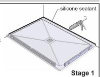
Once the walls have been tiled but before the enclosure is installed, the tiles must be silicone sealed to the tray all of the way around in one continuous bead.
