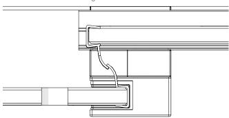
The PLEXRF-027 seal fitted to the door will need notched top and bottom in order to clear the top rail and the bottom slider guide. The top notch does not need to be cut all the way to the hard plastic, only enough to clear the rail. Dimensions shown on images. we recommend using scissors to cut seals.
